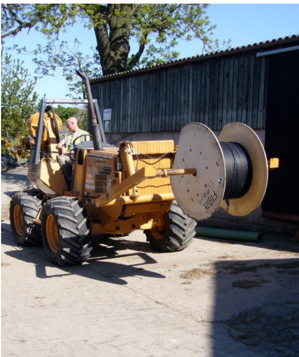
Tony Swidenbank's mole plough arrives and we put the fibre on its reeler.
