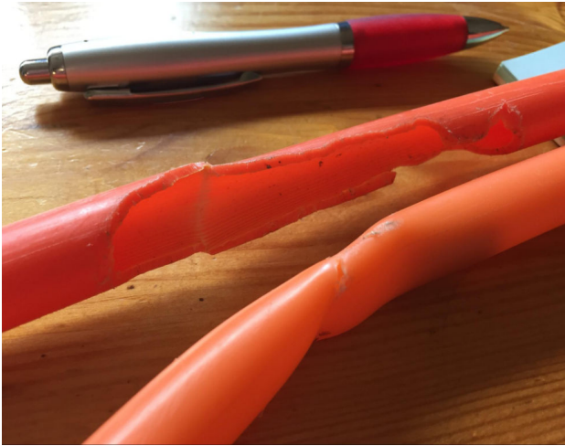
The damaged duct caused by rodents.
