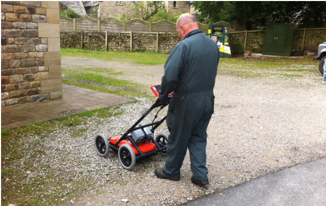
Tom using the ground radar to locate underground services at Abbeystead village hall.
