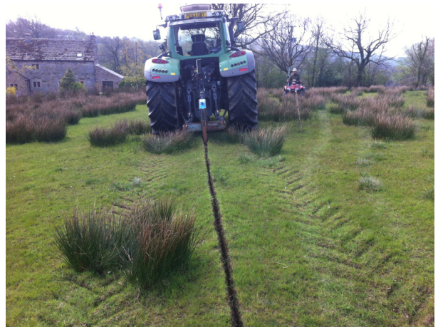
A tractor mole plough in action.
