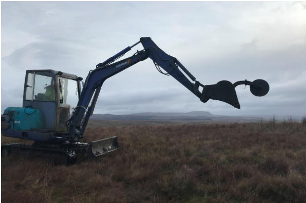
The disc cutter. It didn't work very well on the tough fell.
