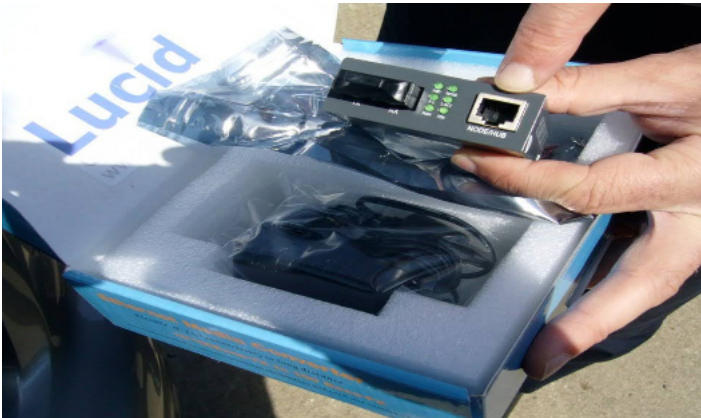
The media convertor that would turn the farm wifi via ethernet into light to feed the fibre to Julie's house.
