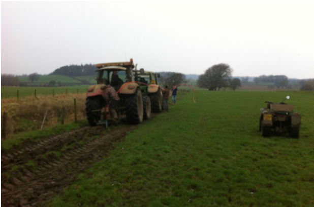
Two tractors pulling the drag mole plough.
