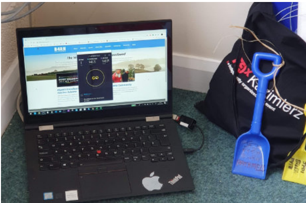
The first speed test at the old school in Rathmell. 940 Mbps symmetrical.
